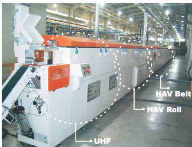
Microwave vulcanization production line and process technology
