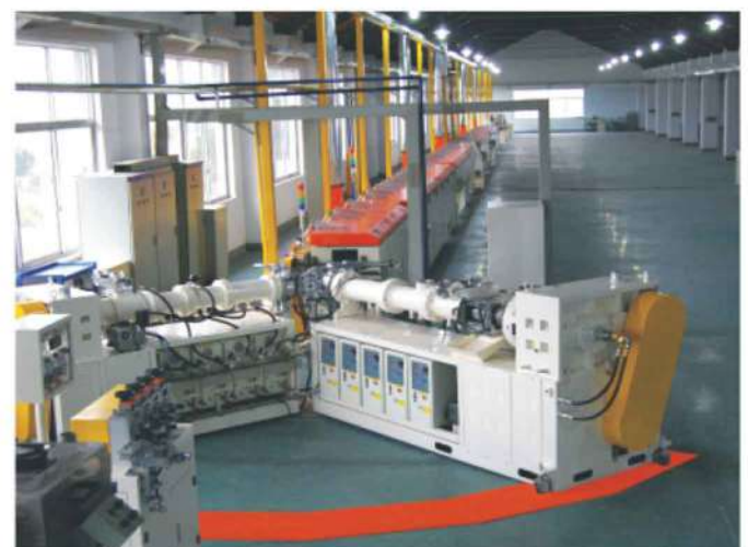
Three (four) compound microwave vulcanization equipments and process
